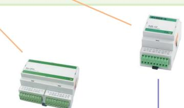
IEX is proprietary low level network based on CAN (Controller Area Network) bus protocol. IEX protocol uses all advantages (reliability, speed) of CAN bus to connect different expansion units to CyBro-2 controller. Expansion modules have unique network addresses and when they are connected, modules are detected automatically - so there is no need for DIP-switch addressing.
